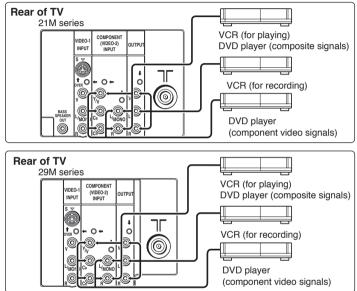
When you use VIDEO-1 INPUT, you should choose to connect S-VIDEO or video input. If S-VIDEO connector and video input are connected at the same time, no picture displays on the screen and the message "PLEASE DISCONNECT VIDEO-1 CABLE!" appears. In this case, you should disconnect either S-VIDEO or video input.
